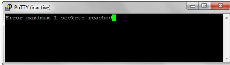
Inactive connections will timeout after 30 seconds by default. Disconnecting from the socket is done by sending the `bye` command to the lamp. The lamp does not send anything in response and just closes the socket.
