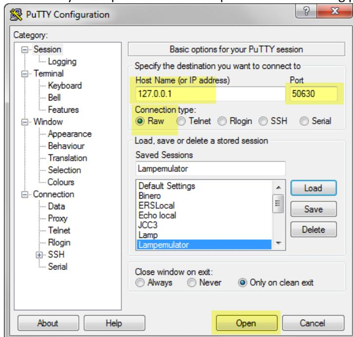
The host name is the IP address of the lamp you are connecting to. In this document an emulator is used which is why the loopback address 127.0.0.1 is used.
